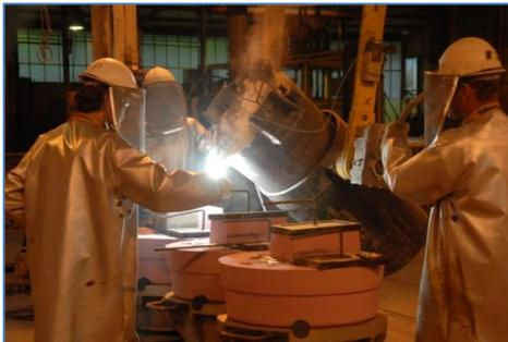
Molten metal is poured into the mould on a **low pressure casting** station via a complex feeding network that ensures the integral filling of the mould.
